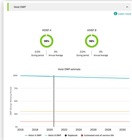
Hoist DWP is the calculation of the remaining service life of the hoist and an indication of the remaining fatigue life of the machinery components. When the DWP value approaches zero, the hoist should be overhauled or replaced.
